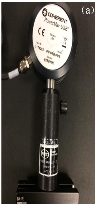
Figure 2.4 The device to detect the laser power; (a) the model of PowerMax USB; (b) the interface of PowerMax.
